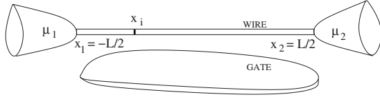
FIG. 1. A quantum wire with an impurity adiabatically coupled to metallic leads. The leads are held at different chemical potentials \mu_1 and \mu_2 .
